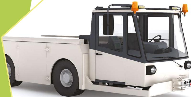
Featured is the NEW FB150E full electric conventional tractor. Available in 12-15 tons weights, with four wheel drive and two wheel steer. The new FB150E is also equipped with the high quality Kalmar Motor cabin, which has central drive position for safety as well as the swivel seat for optimal operational safety and driver comfort. Learn more at [www.kalmarmotor.com](http://www.kalmarmotor.com)
